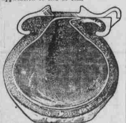
Illustration shows how the tube may be caught underneath bead of case. This may occur from putting too much air in the tube before application or from not using care to keep tube away from rim until beads of case have been properly engaged in channels of rim. This may also occur from using a tube of wrong size. For example, a 4 1/2 inch tube in a 4 inch case. If flap works out of position when the tire is being applied to rim, tube may be injured by flap or bonds of case. When a tire is inserted soft, there is a tendency for the beads to lift up at the toes due to the internal pressure and weight of car and sometimes permit tube to work under bead. This is aggravated when the tire has been constantly ridden soft and beads have been cut and broken by rim.
