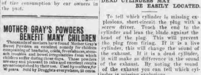
the exhaust. If it is a dead cylinder, it will make no difference in the sound of the exhaust. By noting the sound of the exhaust you can tell which cyl-
