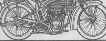
Some New Features Not Embodied In Former Models. 25 per cent greater power motor; oversize valves, entirely enclosed. Foot operated starter with automatic compression control. Motor drive chain and clutch mechanism entirely enclosed.
