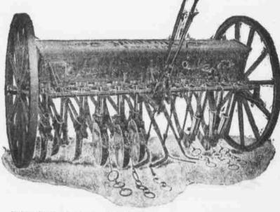
This drill is shown here with the double dises, hoes and shoes on, illustrating the interchangeability of the Monitor. Although out of our entire last season's sales everything but one was the double disc, and that was a souder.
