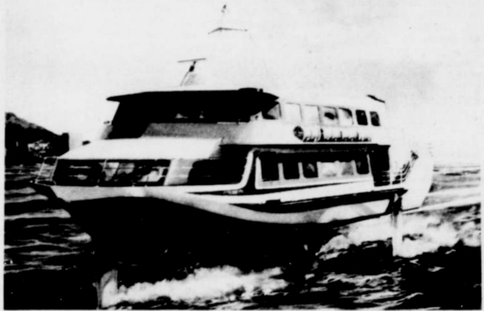
CAPABLE OF SPEEDS of 50 miles an hour over rough ocean water are Boeing Company, Renton, Wash., Jetfoil 929 commuter boats, being manufactured of Northwest aluminum. Ten of the 90-foot vessels, capable of carrying up to 250 passengers are being built, the first to be completed in mid-March. Some 1.2 million pounds of aluminum from the
