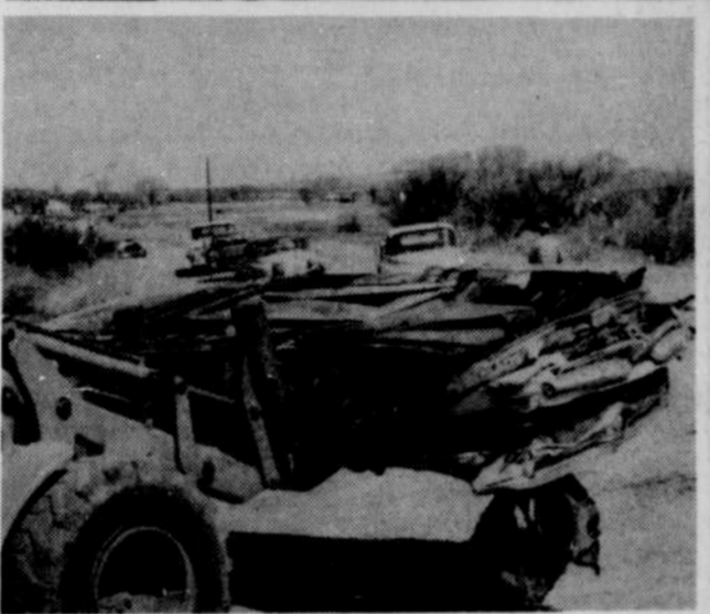
The top photo shows the crusher at work. In the bottom photo the loader is taking away four car bodies in one bundle, after being crushed, and ready for shipment.
