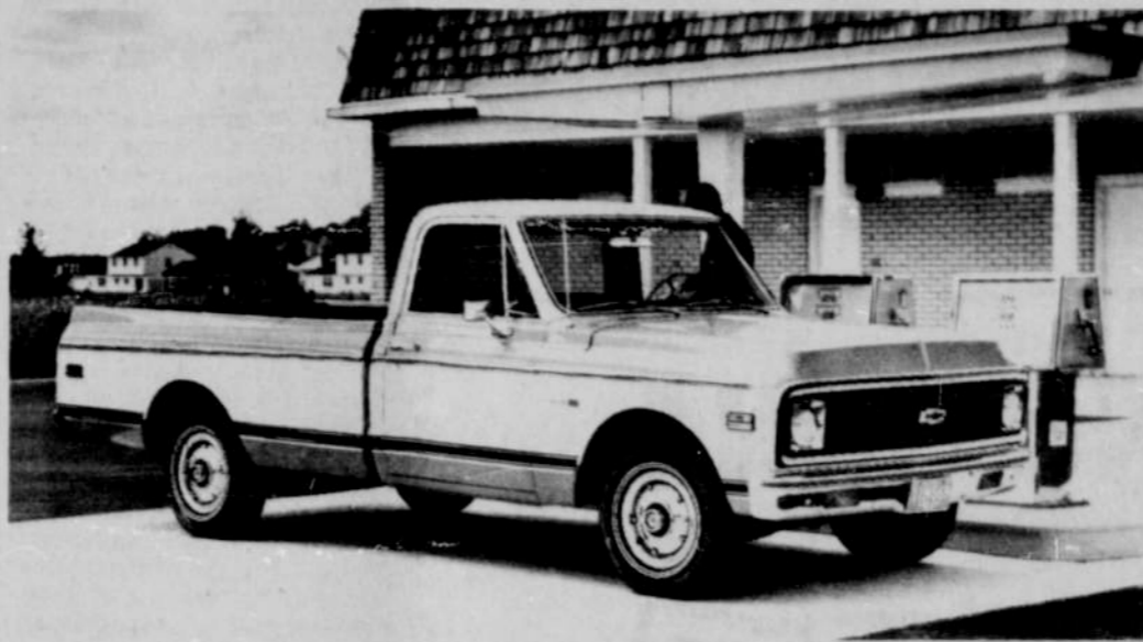
Front disc brakes as standard equipment on all but Chevy Vans highlight the many improvements in the 1971 Chevrolet light truck line. The disc brake system has a proportioning device for more balanced braking between front and rear wheels. Also new are a more massive looking grille, improved cab seating and ventilation, and more powerful headlamps. All engines will operate on the new lower lead fuels and meet required Federal emission standards.
