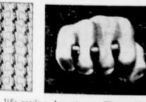
brakes, tread ribs of your tires tend to compress into a smooth, slippery surface. That's because the ribs squeeze together under pressure - like the edges of your fingers when you make a fist. Tread loses its vital grip on the road ... and you skid!
