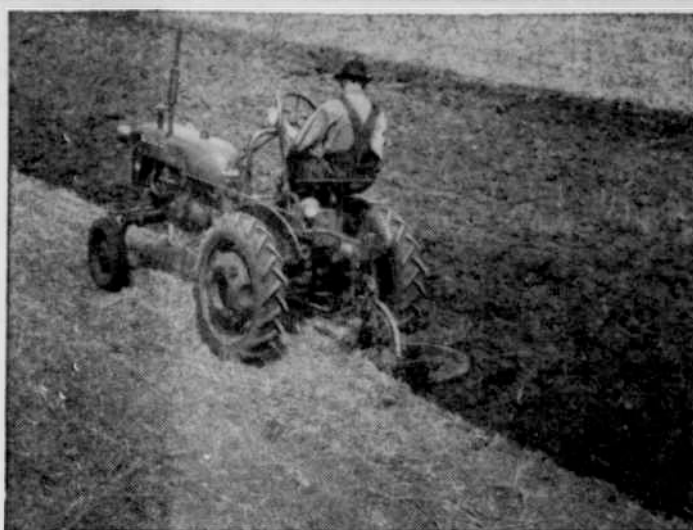
FARMALL CUB FOR PLOWING —International Harvester's new Farmall Cub tractor offers the small-acreage farmer the advantage of complete, low-cost mechanization. It is designed to handle all field and garden crop operations. The above view shows a Cub-193 moldboard plow turning a 12-inch furrow.
