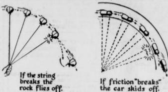
The above illustration is self-explanatory. It shows the part that friction plays in causing an automobile to skid. It shows the need for greater caution on curves. It is a practical lesson in the art of Sportsmanlike Driving.
