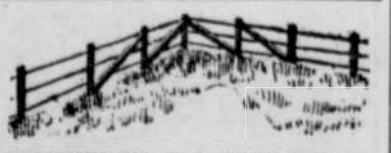
BRACING FOR THE CORNER POST.
