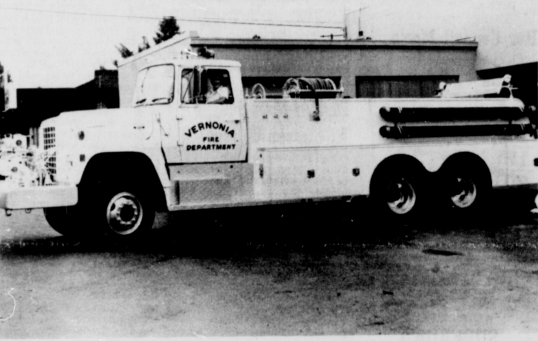
RUSS VINEYARD couldn't resist trying out the new Vernonia Fire Engine following its delivery Monday. The approximately 35 foot long white machine was built by Western State Fire Apparatus in Cornelius. Constructed on a Ford chassis, the vehicle is able to carry 1500 gallons
