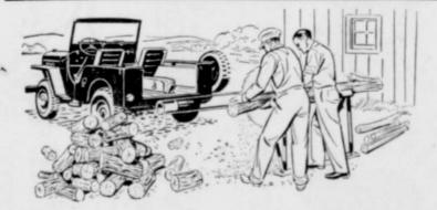
. . . for operation of belt or shaft driven equipment will develop up to 30 h.p. for use of welder, generator or air compressor with the new
