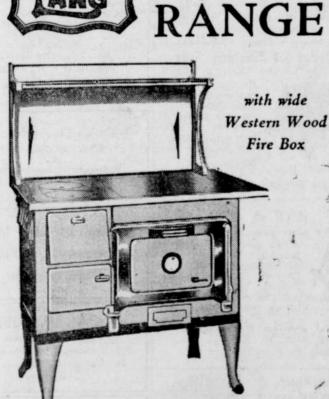
A distinctly different wood range, not too large, has a wonderful baking oven, 28 inches by 18 inches. The double preheat draft solid bottom firebox consumes the charcoal waste and eliminates the necessity of an ash pan. Firebox is 21 inches long, 8 inches wide and 8 inches deep. Burns 18- to 20-inch wood. Body of Zincoat metal. Furnished in white or
