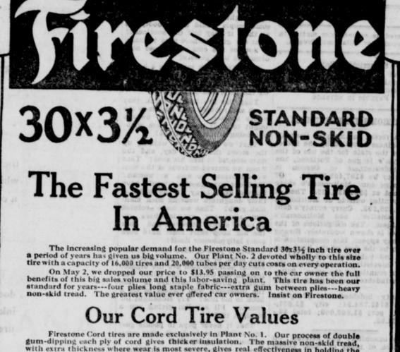
gum-dipping each ply of cord gives thicker insulation. The massive non-skid tread, with extra thickness where wear is most severe, gives real effectiveness in holding the car against slipping and adds many extra miles of service.
