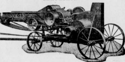
It has an all steel, Lowdown frame and steel truck. It has a malleable cutter head, malleable cutter bar, six fan blower, Alfalfa meal making attachment, and positive safety device, which marks an unusual advance in the building of ensilege and feed cutting machines.
