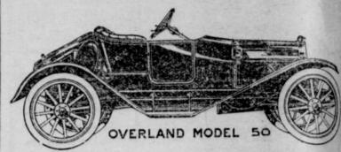
Two passenger torpedo body 20-horse power, transmission. planetary.
