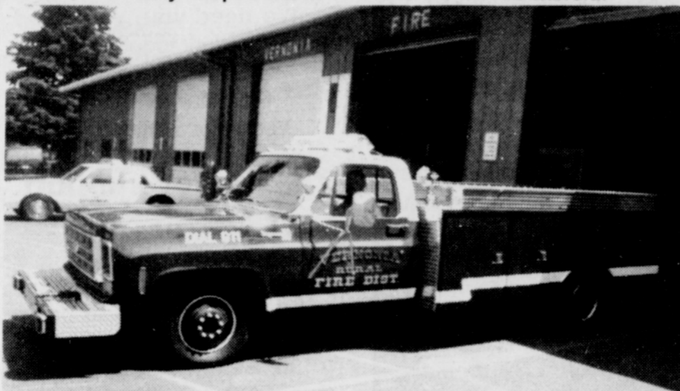
A new first response foam and rescue unit for the Vernonia Rural Fire District utilizes the chassis of an old ambulance.
