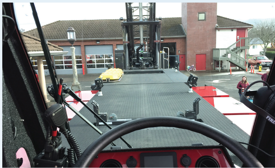
At the front of the quint, the driver communicates with the operator in the rear to steer and operate the ladder.
