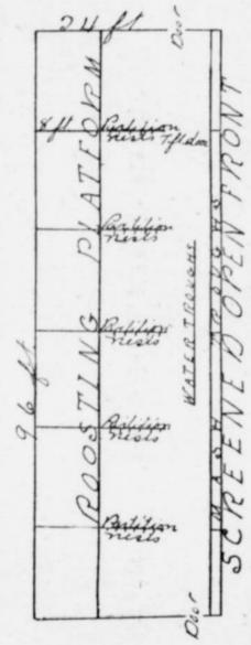
partion running within seven feet of the open front, extending clear to the ceiling. The object of this partition is to break the draft which would be created in a house the length of this one in which there were no partitions. The open space of seven feet is fitted with a door which may be closed at light, in which there is a small hole through which the hens may pass at milk twice a day. will. Mr. Smith's own words will ex- . plain the object of this arrangement to the best advantage.
