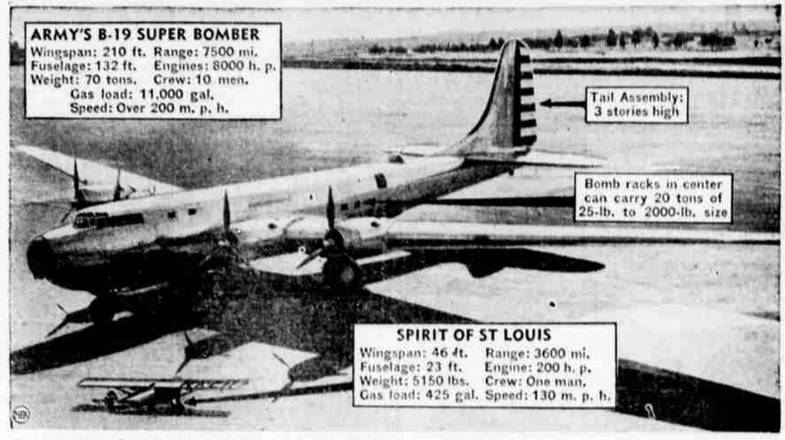
Just 14 years to the month after Charles Lindbergh made his historic non-stop flight to Paris in the Spirit of St. Louis, the U. S. Army's B-19 super bomber is getting its first tests. Pictorial shows how the monoplane of 1927 compares with the giant four-motored bomber of 1941. B-19 could make flight Lindbergh made, and come back again without stopping.
