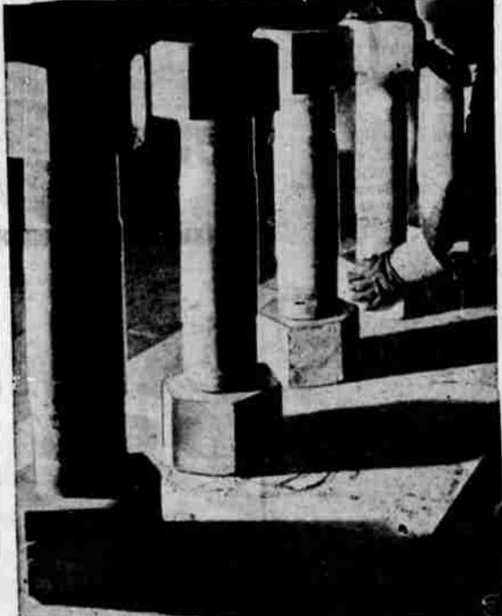
Striking photo is made as workman at East Pittsburgh Westinghouse works coats 315-pound stud bolts with protective compound. Bolts will join sections of a steel shaft of a giant generator.
