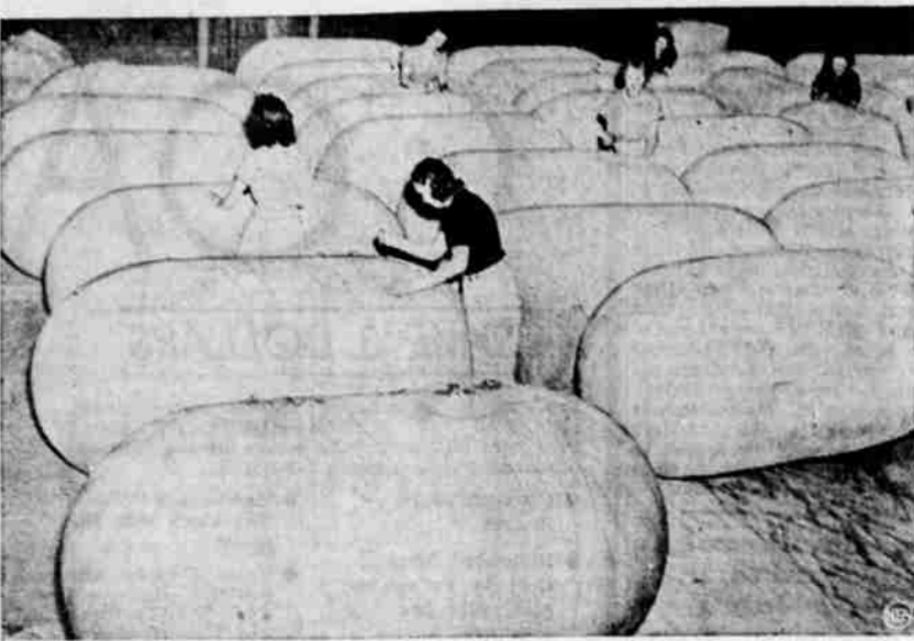
These are flotation bags designed to save Uncle Sam's land planes and their occupants if forced to descend on large bodies of water. They're being assembled at Goodyear's Akron plant for immediate use.
