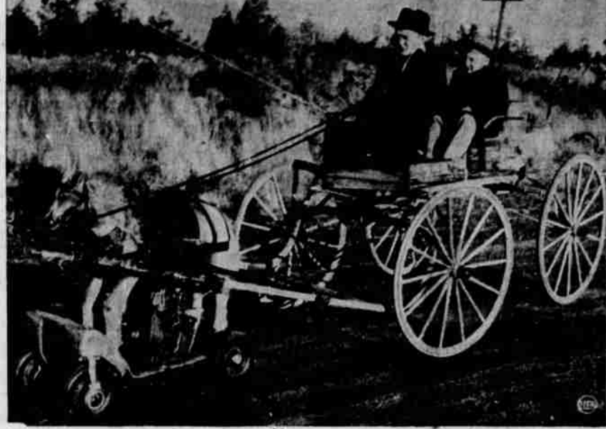
From parts of a cream separator, a washing machine, sheep shearing gear, lawn mower and a Ford, Roy Sheldon, Redmond, Ore., mechanic, made this one-hoss gadget. The horse pulls the wagon at 15 mph and runs all day on a gallon of gas. Roy steers with the reins, the horse's head turning the wheels. Like modern automobiles, the horse has knee action, and gallops along as it pulls the wagon.
