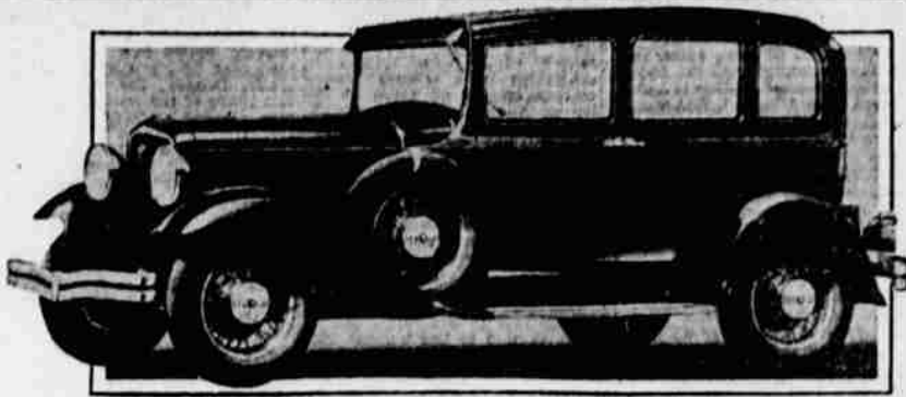
The New Studebaker Six Regal Sedan for five with Free Wheeling. Brilliant 70 horsepower engine. 114 inch wheelbase. Six wire wheels and folding luggage grid are standard. Price is $995 at the factory.
