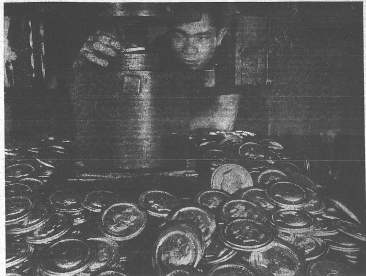
Louis Santiago places a bronze 1965 Inaugural Medal between dies on a 1,000-ton press at Medallic Art Company in New York. At right, after four strikes, a medal is examined for detail of impression.
