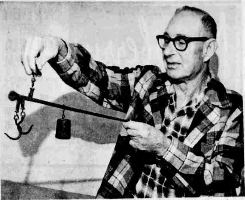
MIGHTY OLD — Brothers John, Hans and Thomas Minkler, came to America from Holland in 1709, bringing with them this hand wrought iron scale. Jack Minkler of Klamath Falls now owns the relic. His father, Frank, and later his children were weighed on it. Rules differ on each side of the beam. One side weighs up to 45 pounds, the second to 12 pounds. The three hooks are held by pins. Jack Minkler, a retired logger, came here from Eugene in 1953. The family home is at 234 Martin Street.
