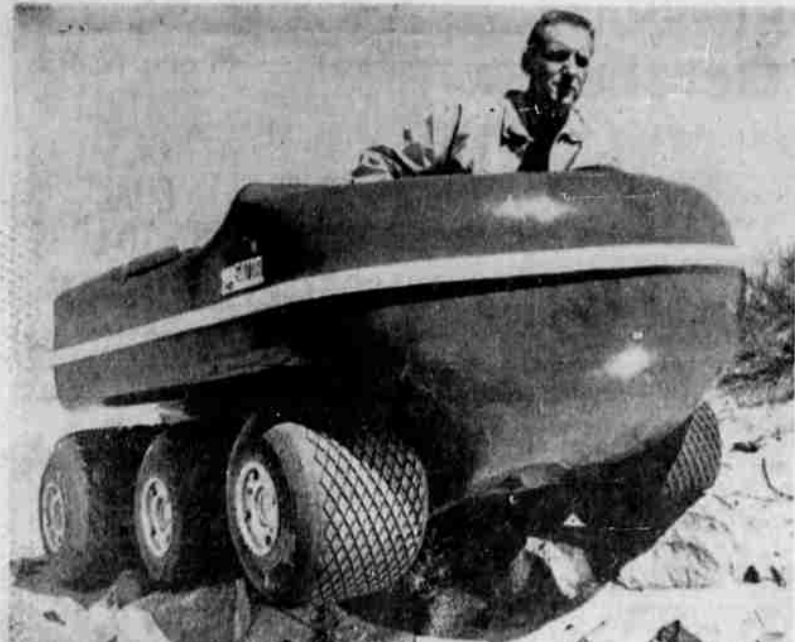
TEST RUN — An engineer puts the amphibious "Terra-Gator" through its paces recently in New York. The vehicle, with its six-wheel drive and fibre-glass body, gets its traction and much of its buoyancy from huge "Terra-Tires" developed by Good-year. The unique vehicle is manufactured in California. —UPI Telephoto
