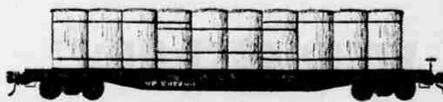
New "floating-load" tie-down technique can speed loading and reduce shipping costs for other forest products besides finished lumber. Here, twenty huge rolls of paperboard ride secure and protected on one of S.P.'s new 53-foot, Oregon-built flat cars.
