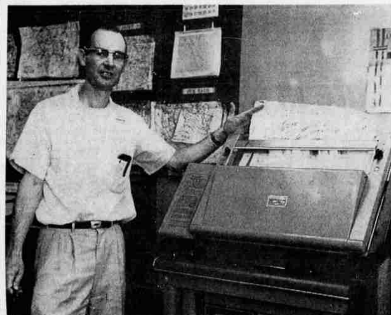
WEATHER MAPS — Jim Rawles of the U.S. Weather Bureau office at Kingsley Field, holds a weather map coming out on a facsimile machine from Washington, D.C. The Weather Bureau office here receives an up-to-date map each six hours showing conditions all over the country.
