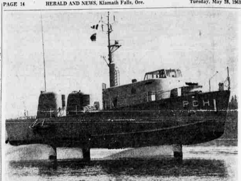
FLYING HIGH — The U.S. Navy's first patrol craft, Hydrofoil PCH-1, demonstrates the lift capacity of her wing-like foils under the hull. The craft is designed for speeds over 50 miles per hour, and will be used as a submarine chaser. Built by the Boeing Company, the High Point will lift as high as six feet off the water on the foils.
