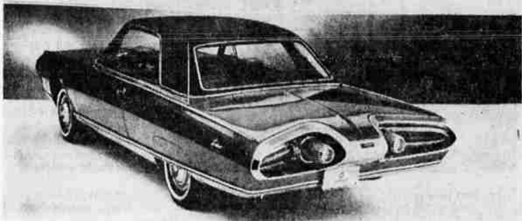
TURBINE AUTO — The world's first family-size passenger car specifically engineered and designed for turbine power is shown here as unveiled recently by Chrysler Corporation. Fifty of the turbine cars will be built and tested in various parts of the country to test consumer reaction and acquire drive experience.
