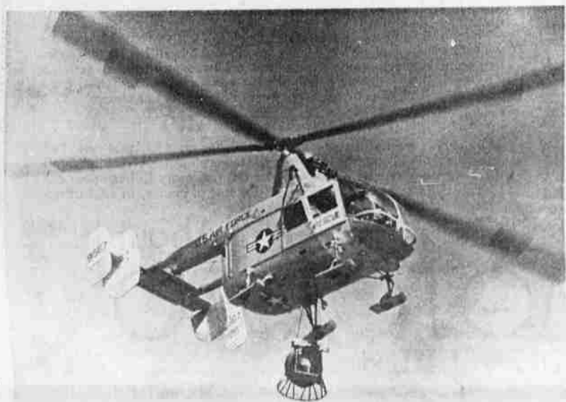
SPECIAL FIRE FIGHTER — Quick fire control is obtainable at Kingsley Field in remote areas with the use of this helicopter which carries a giant-sized foam fire extinguisher underneath. It sprays out foam and the copter blades spread it over the fire.
