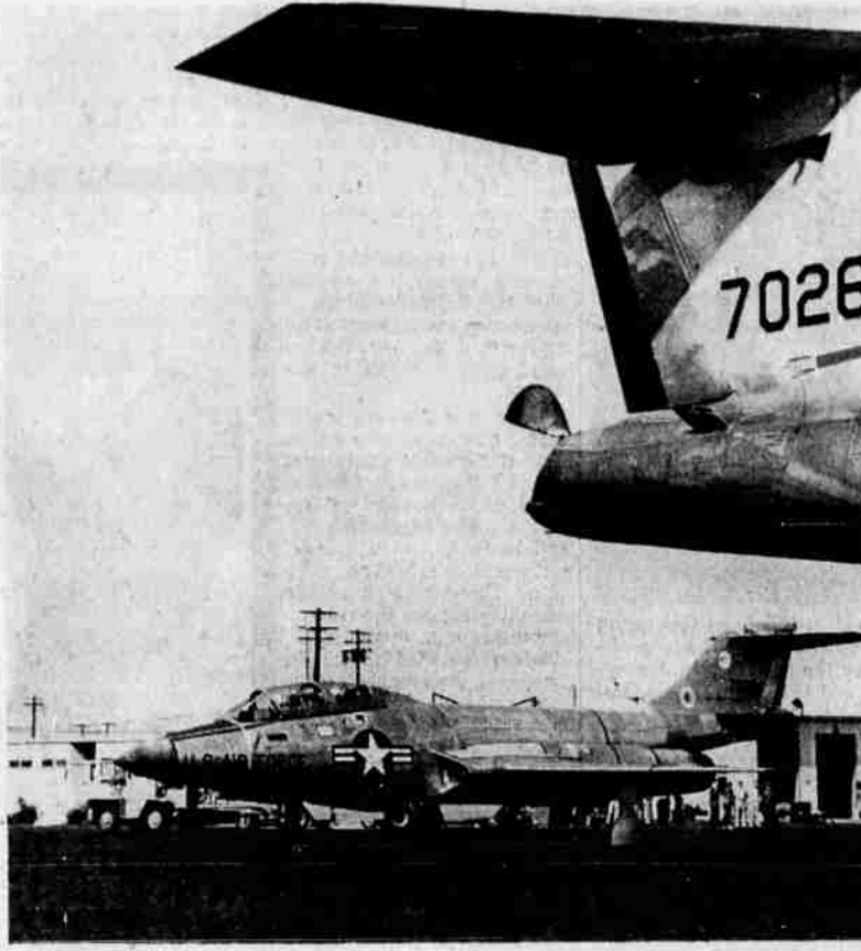
TAXIING IN — One of Kingsley Field's F101-B "Voodoos" taxis into the parking area after landing on a return flight from McChord AFB, Wash. Visible at right is the door at the rear of the aircraft from which a "drag chute" pops during landing to help slow the huge aircraft. Crews from the 322nd Fighter-Interceptor Squadron flew the planes home. Ground crews and maintenance specialists from the 408th Consolidated Aircraft Maintenance Squadron also returned to Kingsley this week.
