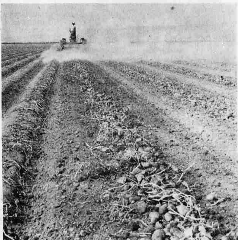
A TWO ROW digger is busy at work laying the potatoes on top of the ground where they can be gathered. The telltale clouds of dirt mark the digging operations each fall in the potato fields of Basin.
