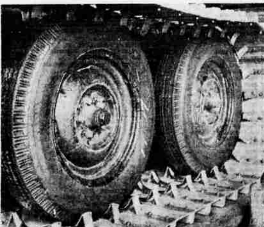
TREADS OF THE OLSON snow cat run on six wheels, the chain driven back wheels, the center idlers, and the front set.
