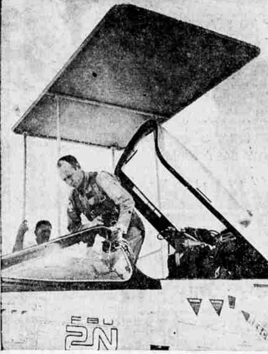
JET UMBRELLA —An innovation in the flight test line at Chance Vought Aircraft's plant in Dallas is this umbrella for Crusader jet cockpits. It is designed to protect the pilot from the Texas sun until the plane's air conditioning unit is working. The umbrella is mounted on a mobile dolly and is easily moved after use.
