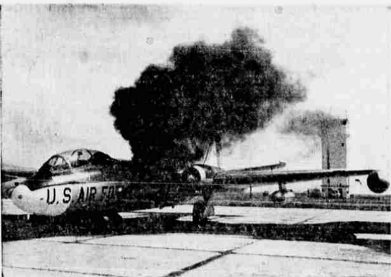
NO FIRE, but this Martin B-57 twin jet bomber turns out a cloud of black smoke each time the engines are started. It's a black powder cartridge fired to start the engines. The B-57 is powered by two Wright J-75-5 turbojets which give it a speed in excess of 600 m.p.h. and a ceiling over 45,000 feet. The bombers have a range of over 2,000 miles and carry two crewmen. A flight of seven of these bombers spent a portion of the week at Kingsley Field, departing after midweek for their home in New York. — Photo by M.Sgt. Charles Bennett
