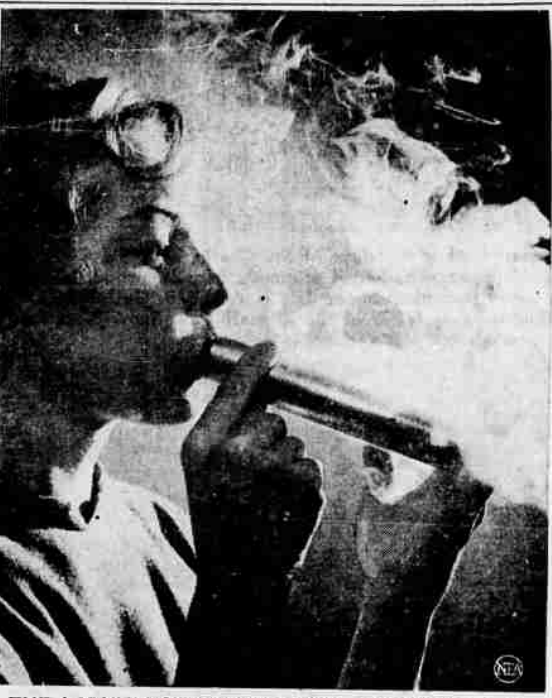
THE LADY'S NOT FOR BURNING—Joan Gunderson exhales cigarette smoke through microscopic pores of a length of steel pipe made from fine, flattened steel wires. Called Poroloy and made in Madison Heights, Mich., the pipe will be used where heat is a problem because the pores can allow a coolant to pass through.
