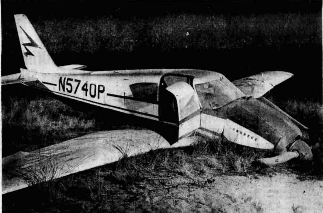
THIS PIPER COMANCHE was extensively damaged Friday night when it crash landed just after takeoff at the north end of the municipal airport. Anton J. Steinbock, veteran flyer and owner and operator of Klamath Aircraft Service, was piloting the plane when the engine failed on takeoff.
