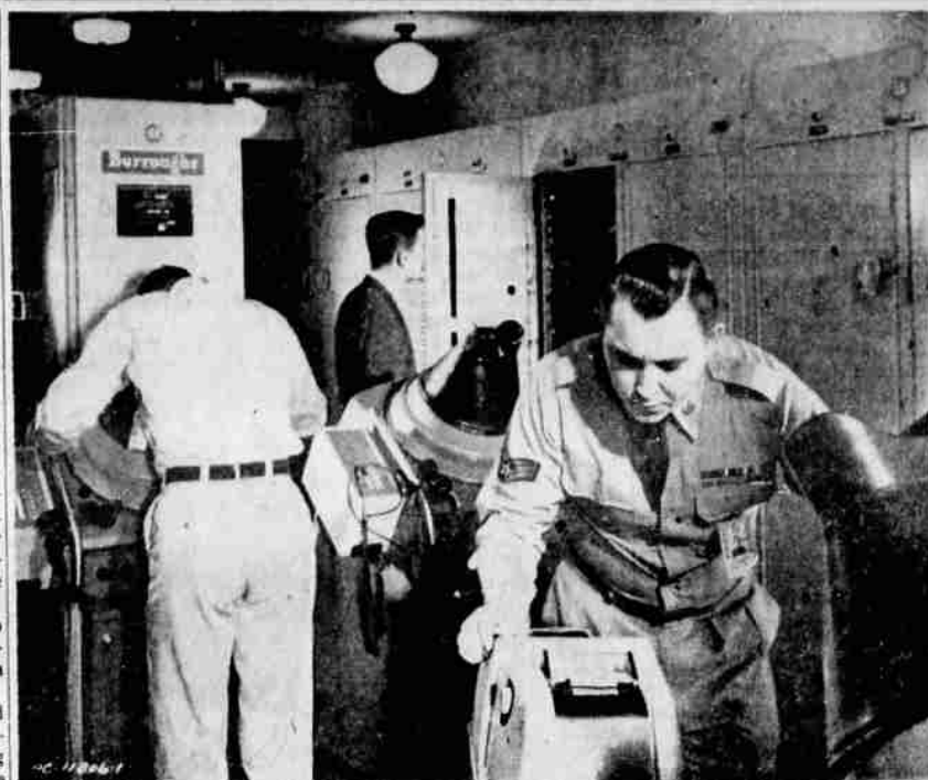
INSTALLATION of a huge data processing system in Klamath Falls signifies the community's entrance into a continental air defense role. Here, unidentified U.S. Air Force technicians and a Burroughs Corporation engineer put the machine, titled AN-FST-2 through its paces. The "T-2," chief building block for SAGE, is a duplexed data processing system which processes friendly and enemy target information picked up by radar in outlying sites and transmits the information to direction centers. There it is coordinated with target information from other sites to alert defense weapons, if necessary.
