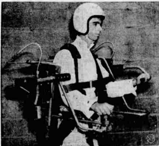
OVER THE MOON? —Engineer Richard G. Peoples demonstrates personal rocket for the infantryman of the future. Called "Aeropak," the plumber's nightmare would allow soldier to jump over ravines, rivers, mine fields. Angle of liquid rockets is controlled by left hand while throttle in right hand controls speed.
