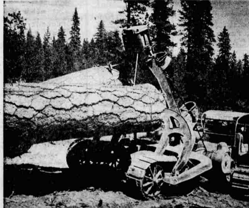
THE NEW TYPE of log handling, being done by modern tractor-drawn equipment is shown here, easily moving a Ponderosa pine log. Industry has also progressed to a high degree of forest management as represented by its Tree Farm program in which the fifty millionth acre will be enrolled this year. This picture from the files of the Western Pine Association.
