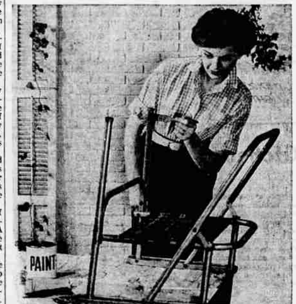
Exterior enamel in a bright color reconditions an aluminum chair for another summer's outdoor service. Set upside-down on table and paint underside first, to speed your painting time.
