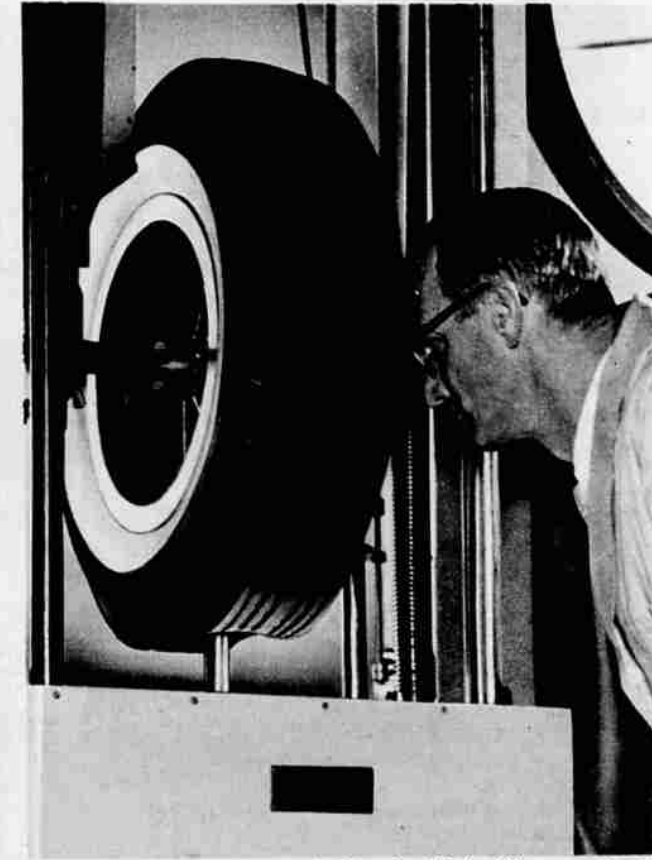
IN TESTS Atlas gives them the most thorough going-over...like this test (shown in picture above) to check tire carcass strength.
