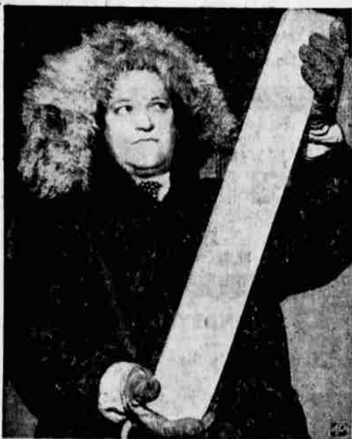
ICE WITH A PAST — Physicist Theodore Bulkovich, at Wilmette, Ill., Army center, holds ice core taken from Greenland icecap. The ancient core may hold bacteria and atmospheric bubbles dating back to year 1100.
