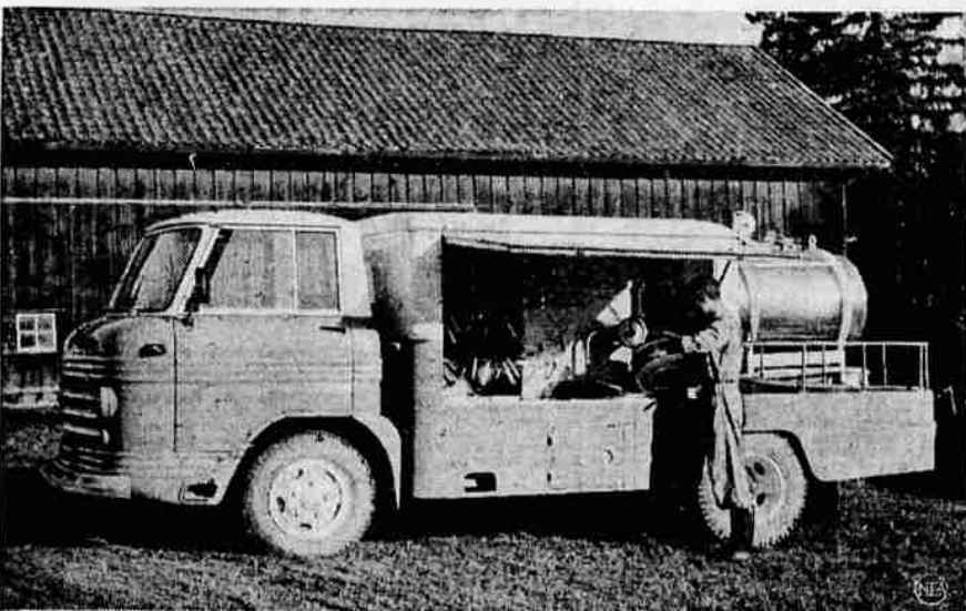
MILKING TRUCK — This mobile milking unit has been used experimentally in central Sweden where farms are far apart and distant from the dairy. Eight farms with a total of 65 cows are serviced by the truck which is modeled after units used successfully in Holland and Germany. It's equipped with six milking machines, washing machine, water tank, water heater and three milk tanks holding 160 gallons each. There are also two vacuum pumps, an electric motor and a gasoline-powered generator for farms without electric current.
