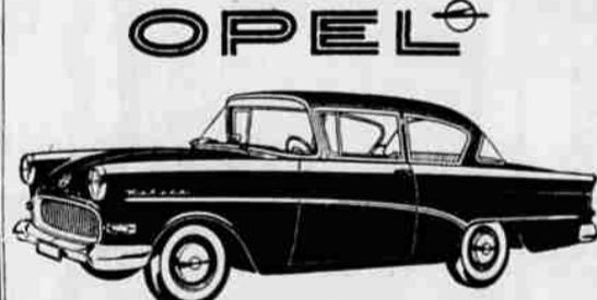
OPEL OLYMPIA REKORD SEDAN 56 horsepower at 4400 rpm • 90.8-cu.-in. displacement • 7.5-1 compression ratio • Curb weight 1995 pounds.
