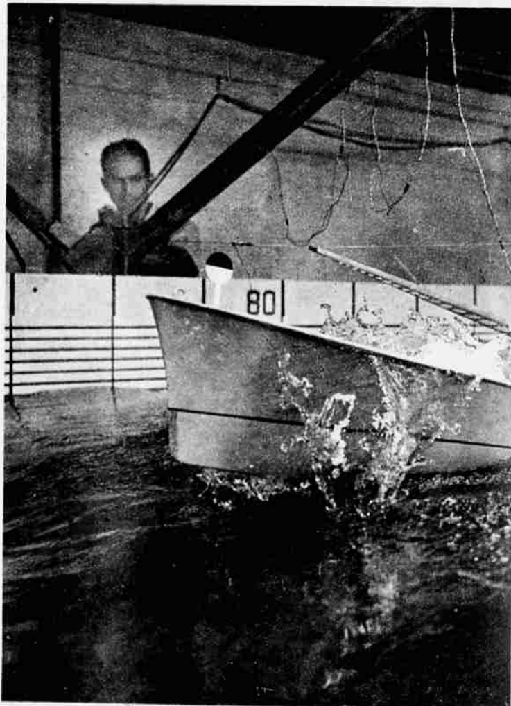
The performance of this small, graceful hull model of a naval frigate is studied carefully by maritime scientist.
