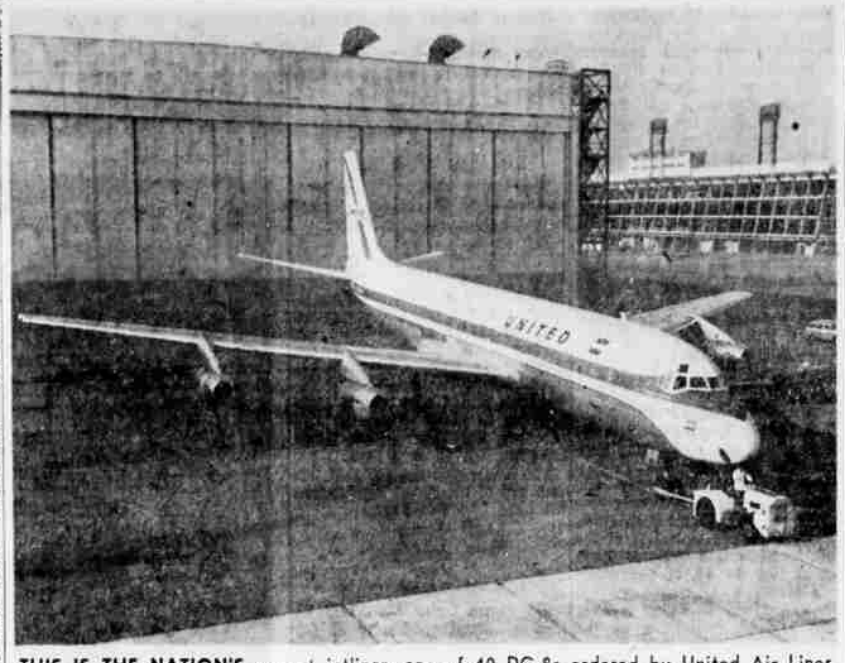
THIS IS THE NATION'S newest jetliner, one of 40 DC-8s ordered by United Air Lines from the Long Beach, California, factory of Douglas Aircraft which will enter scheduled service next summer. The great craft will carry from 116 to 151 passengers. The 575-600 m.p.h. jetliner must undergo months of ground and flight testing. The plane is 150 feet long with a wingspan of 139 feet. It will fly coast to coast in four and two-thirds hours. Cost of the jets is five million dollars. — United Air Lines Photo
